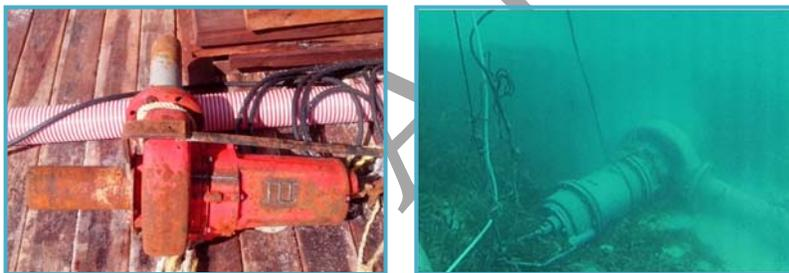
**Figura II\_ 20. Bomba sumergible.**
